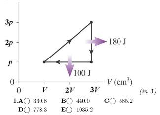
1 pt Find the efficiency of the heat engine.
