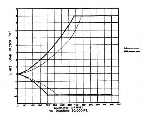
Figure 2-11 MIG-21 and F-4 V<sub>N</sub> Diagram (S-Gp-1)
