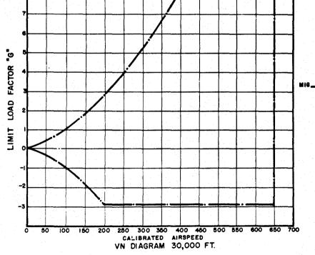
Figure 2-8 (S-Gp-1) MIG-21 V<sub>N</sub> Diagram
