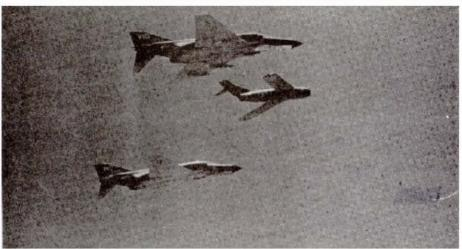
■ The effectiveness of the F-4 radar and radar missile system is substantially reduced when the MiG-17 operates at or below 10,000 ft AGL
